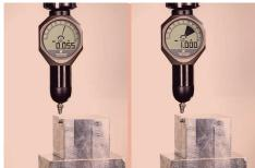
Danger of crash (0 mm till ERR01) When overpassing, the LED warns in red and the black bar builds up clockwise to the right. Shortly before crash (>1 mm), you can see ERR01 on the display..
