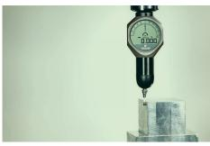
Zero point (precisely reached) When the "O" is reached, the spindle axis is positioned precisely on the edge of the workpiece.
