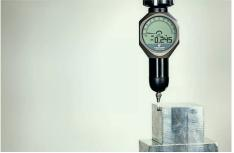
Fiee scale (0,25 till 0 mm) At -0,250 mm, the display changes to the fiee scale and the green LED lights up.
